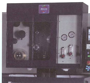
切割銅線承載重量可達10kg Copper wires filler axis is able to load weight of 10 kgs.
